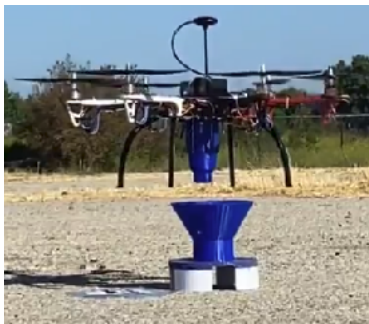
Fig. 16: Testing the precision and accuracy of the PID controller by attempting to land inside the guide cone.
