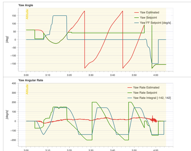
Fig. 11: Attitude control yaw setpoint compared with estimated yaw for the leader drone in the four-drone frame. Top graph is the yaw position, and the bottom graph is the yaw rate. The discontinuous jump corresponds to the graph wrapping around 180 degrees.
