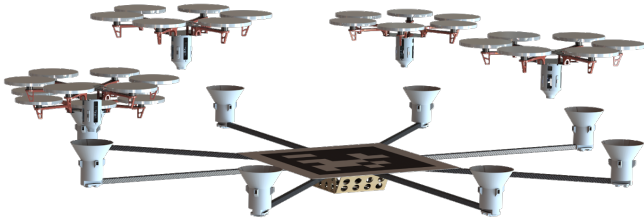
Fig. 1: CAD rendering of the AVIATA frame with the large central AprilTag target and docking joints (peripheral targets not rendered).
