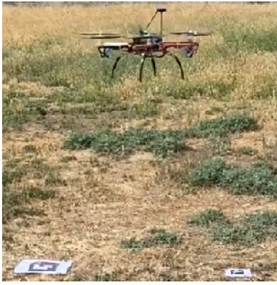
Fig. 15: A drone executing 2-stage docking, currently transitioning between the stages. The central tag is on the left, and the peripheral tag is 1 meter to its right.
